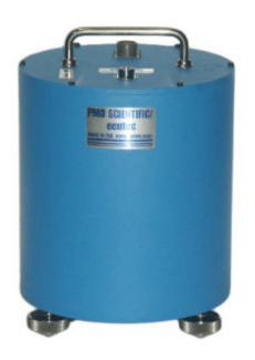
The instrument uses three identical proprietary electrochemical transducers <sup>1</sup> mounted orthogonally along the N, E, and Z-axes. These transducers have many advantages over traditional electromechanical sensors. In particular, they have much larger ground motion-to-voltage conversion ratio that results in a uniquely shaped noise curve that is *essentially flat from several Hertz to the longest periods*.
